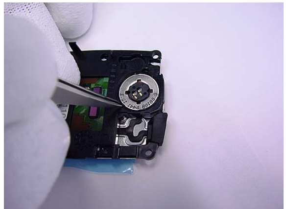
Press the speaker with tweezers out of the UI-Module.
