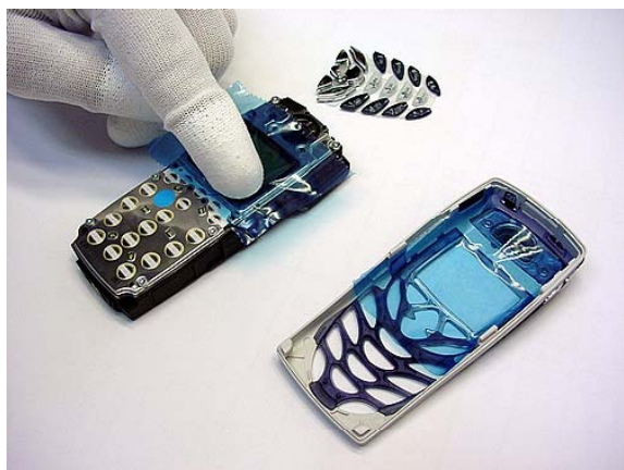
Protect the display with a foil against dust and scratches.
