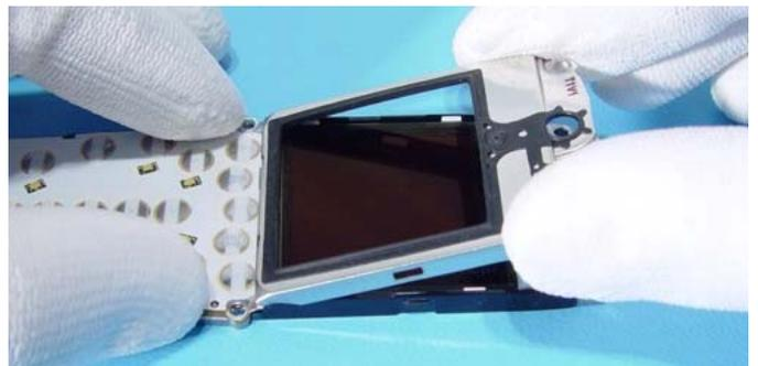
The *Display Shield* is attached with hooks at its bottom side.
