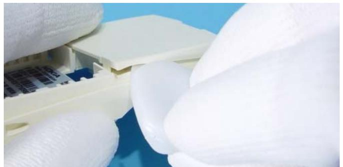
Unlock *Antenna* on both sides with *SRT-6*.
