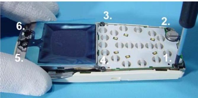
Unscrew the six T6 screws, using the order shown. **For assembly, the reverse order and a torque of 17Ncm have to be used.**
