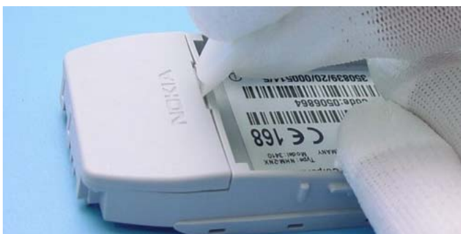
The SRT-6 opening tool is also very helpful, when opening the Antenna.
