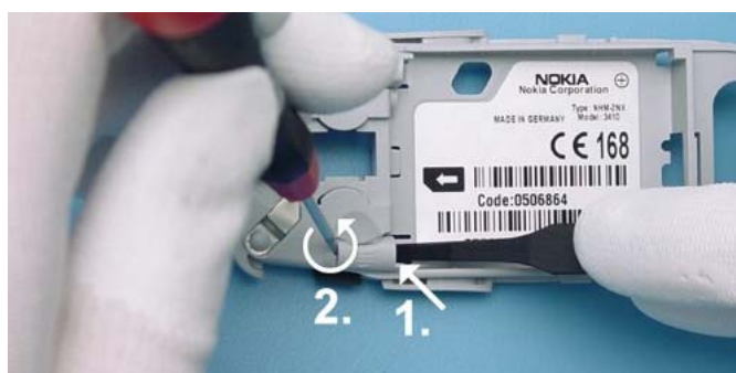
If you need to change the Battery Lock, you first have to press the retaining clips before rotating the straight bladed screwdriver.
