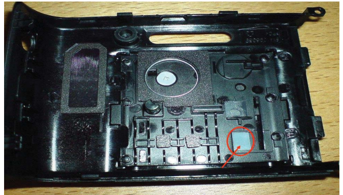
Support pad on the antenna cover.
