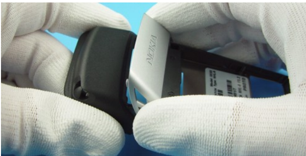
After releasing of the snaps, the Logo Bracket can be removed.
