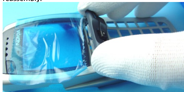
Remove Function Keys. Use always new keys in reassembly!
