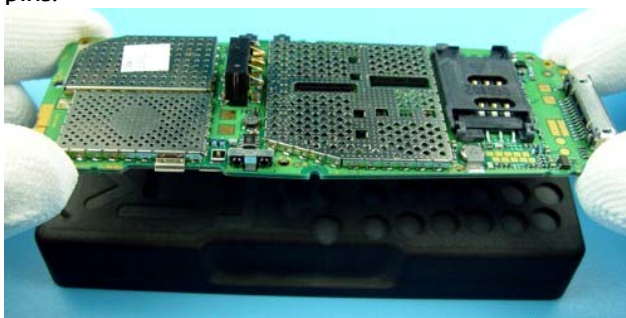
Lift the Engine Module with the new Domesheet from the Jig.
