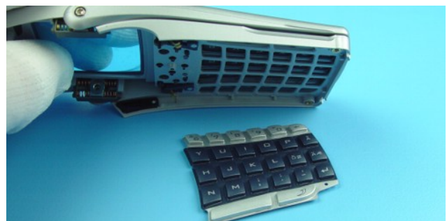
Keymat drops out when turning A-Cover.
